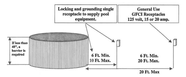
Both receptacles can be on one post between 6 ft. and 10 ft. from the pool wall.
